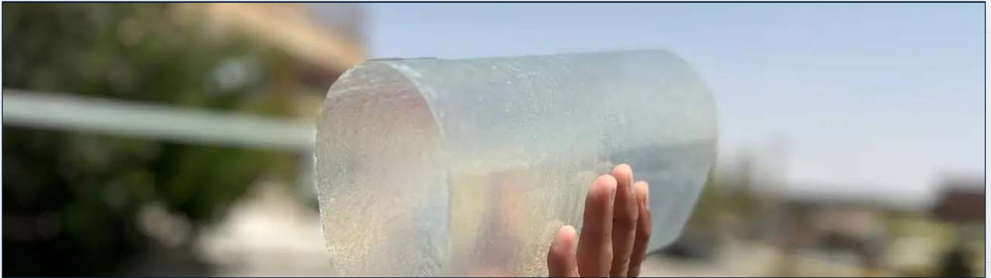
FIG.13-A - Flexible translucent FRP sheet manufactured for industrial and architectural applications.
