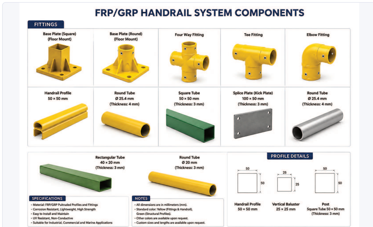
Figure 6 — Components of the composite handrail system: ergonomic top-rail profile, square/round base plate, shaped fittings (elbow, tee, cross), square and round profiles, and kick plate.
